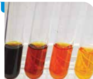
Fig A1 Phenol-sulphuric acid test for monosaccharides
