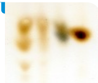
Fig A3 Thin layer separation of monosaccharides
