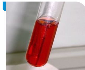
Fig A2 Resorcinol-HCl test for anhydro sugars
